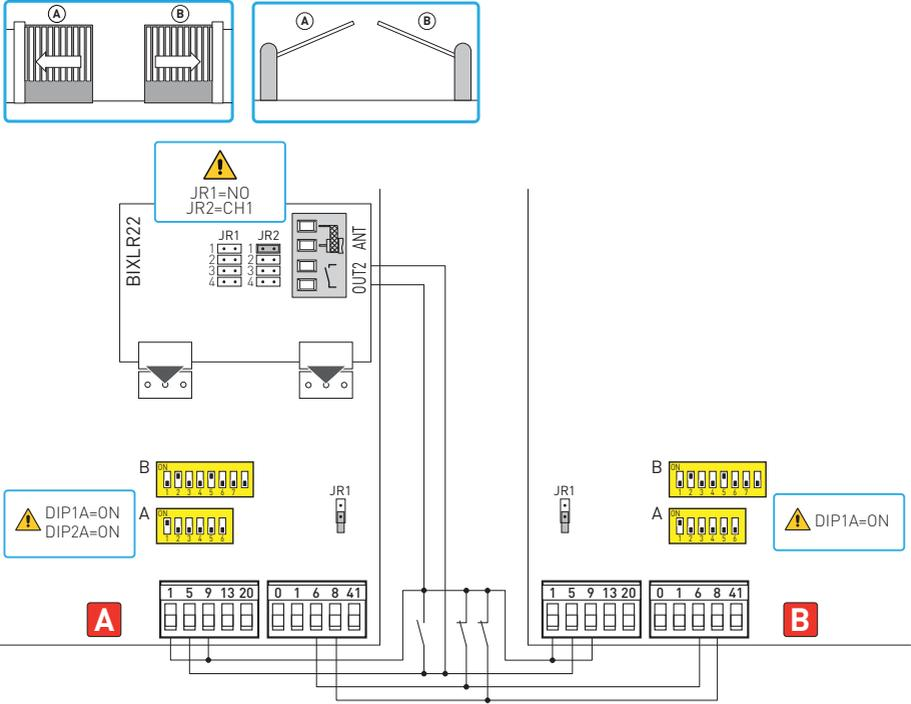
It is possible to command two automations [A] and [B] in parallel with the connections and settings indicated in the figure.
