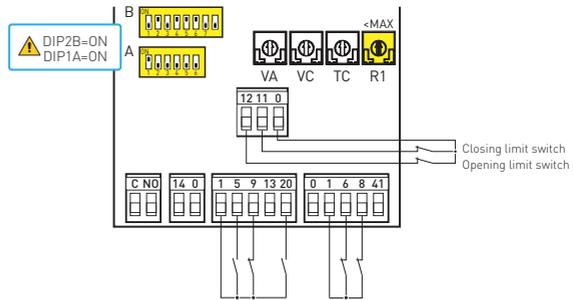
**(Example 2).** The remote control can be used with step-by-step functioning and, at the same time, terminal 5 with opening function by making the connections indicated and setting DIP1A=OFF.
